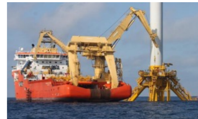
↑ AHTS Normand Sapphire did the tow-out, hook up, and installation of the dynamic cable during Windstaller Alliance's offshore campaign for Saitec – DemoSATH in 2023. This operation turned out to be a very successful campaign proving excellent cooperation with the client and Windstaller Alliance.
